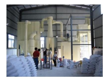
The whole system of Three-ring Micro Powder Mill consists of main frame, reducer, classifier piping device, blower, jaw crusher, dustpan elevator, electromagnetic vibration feeder, and electric switch box motor etc.
